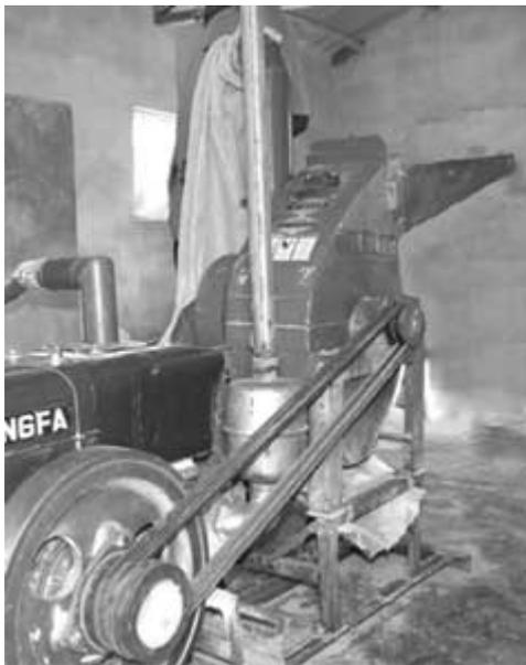
**Figure 3 :** Small forage grinding machine at work in Benin, with a diesel engine, loaded by hand
