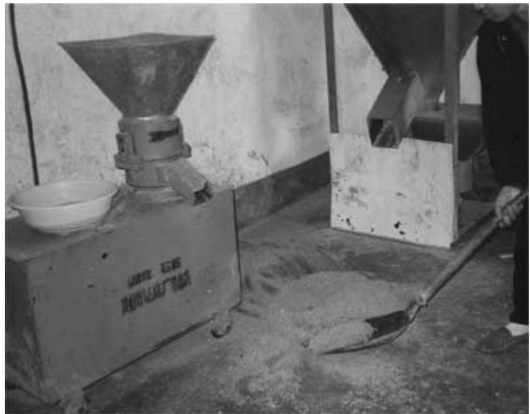
**Figure 4 :** Small pelleting machine at work in China, with an electric engine (protected inside the box below the pelleting device), loaded by hand.
